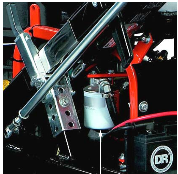
Hydro Fluid Filter – Right Side
