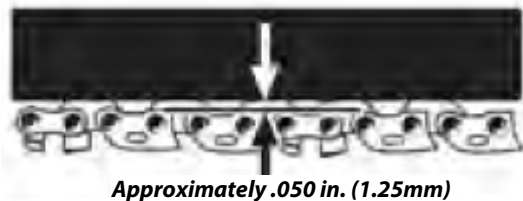
Properly Adjusted Warm Chain
