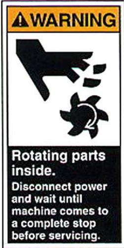
ALWAYS turn OFF the engine, wait five (5) minutes to make certain the flywheel and all moving parts have come to a complete stop and cool, and then disconnect the spark plug wire before servicing the machine. (#091-0381)
