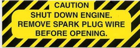
ALWAYS turn OFF the engine, wait five (5) minutes to make certain the flywheel and all moving parts have come to a complete stop and cool and then disconnect the spark plug wire before opening this access panel. (#080-0970)
