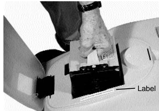
Figure 13. Orient and insert the battery
