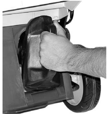
Figure 27. Installing the mulching plug
