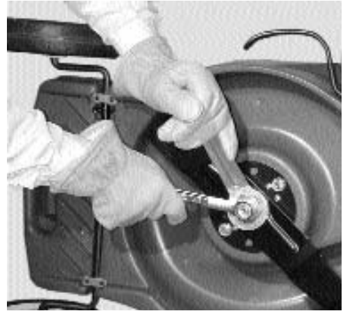
Figure 30. Removing the blade
