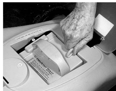
Figure 3. Turn the battery retainer arm
