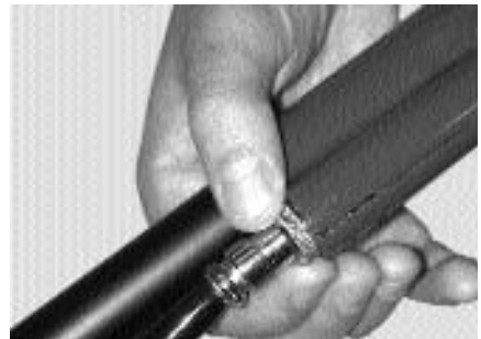
Figure 11. Hand-tighten the locking nut
