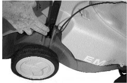
Figure 5. Slide the handlebar fully into the slot on the Mower
