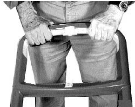
Figure 21. Squeeze the orange control bar
