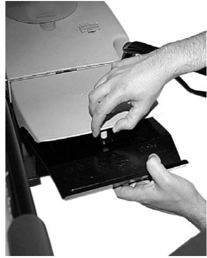
Figure 12. Attach the rear discharge plate
