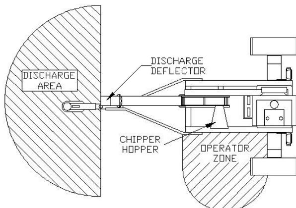
THE EXACT AREA OF DISCHARGE WILL BE DETERMINED BY THE DIRECTION OF THE DISCHARGE CHUTE AND THE ANGLE OF THE DEFLECTOR.
