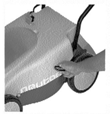
Figure 18. Cutting height lever set to leave your grass 1.6 inches high
