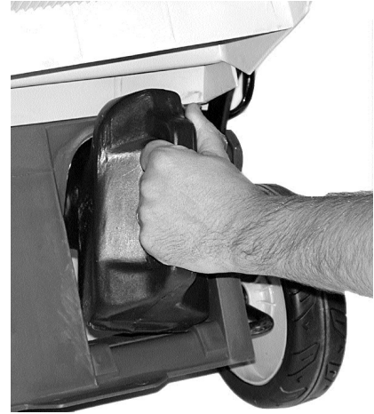
Figure 27. Installing the mulching plug
