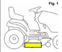
If your discharge opening has a flap (usually rubber or molded plastic), be sure to measure the opening of the DECK, not the FLAP.
