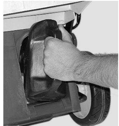
Figure 29. Installing the mulching plug
