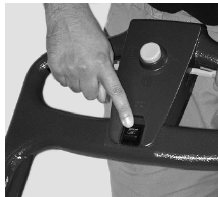
Figure 14. Pushing the Mower/Auxiliary switch to the Mower setting
