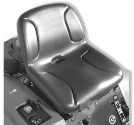
Figure 11. Seat with slide adjuster
