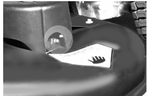
Figure 16. Grease zerk for left blade on the 42-inch model
