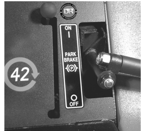
Figure 12. Parking brake set (engaged in the On position)
