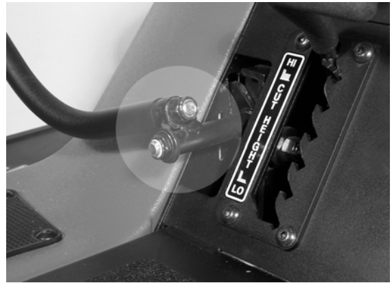
Figure 3. Right drive lever bolt. Both drive levers must be correctly positioned and bolted in place.
