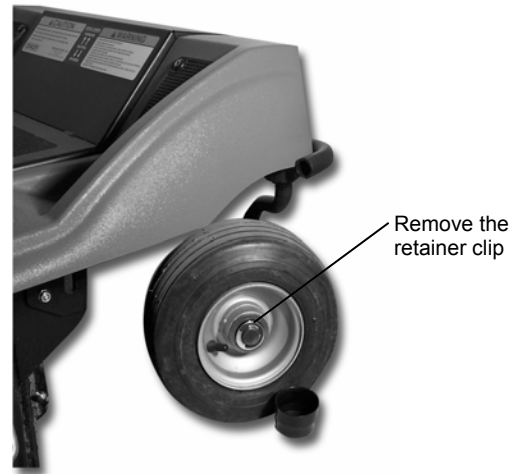
Figure 27. Front wheel with the hub removed
