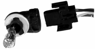
Figure 32. Bulb assembly removed from the wiring harness
