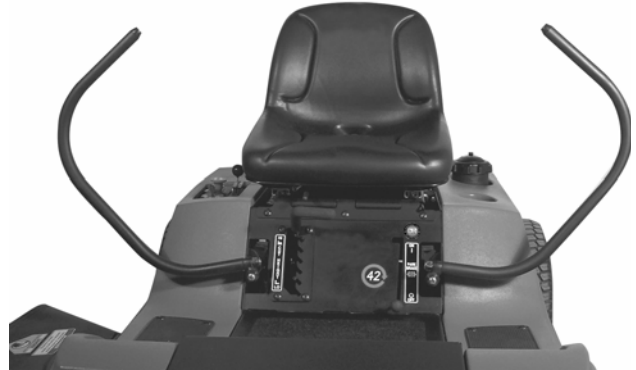
Figure 6. Drive levers swung out, in the neutral position
