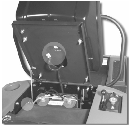
Figure 1. Seat raised, exposing the battery, seat support arm, and the operator presence connection.
