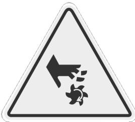
*This label indicates proximity to machine openings with rotating blades inside.*
