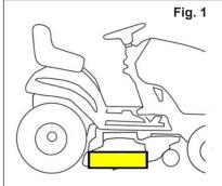
If your discharge opening has a flap (usually rubber or molded plastic), be sure to measure the opening of the DECK, not the FLAP.
