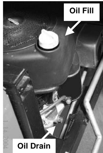
Figure 2: Oil Fill and Drain
