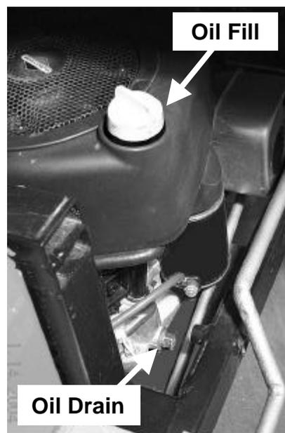
**Figure 11: Oil Fill and Drain**
