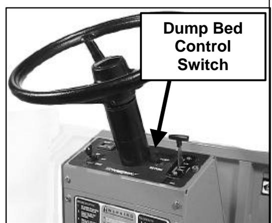
**Figure 6: Dump Control Switch**
