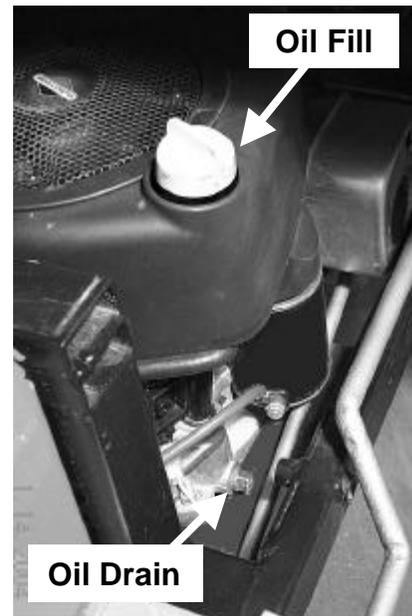
Figure 11: Oil Fill and Drain
