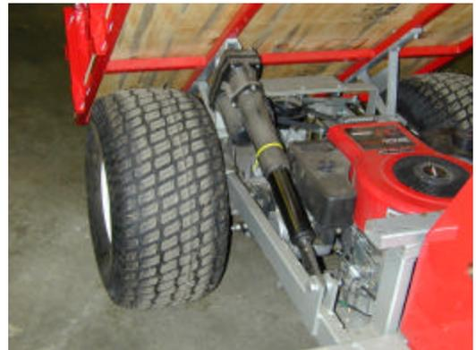
**Figure 7: Electric Dump Mechanism**
