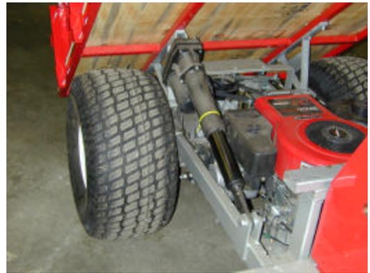
Figure 7: Electric Dump Mechanism
