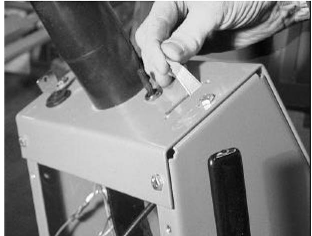
**Figure 21: Preparing To Remove Throttle Lever**
