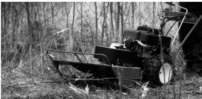
Push Down on Handlebars to Clear Debris
