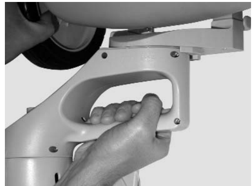
Figure 8. Squeeze the orange handle to adjust the body to trim or edge
