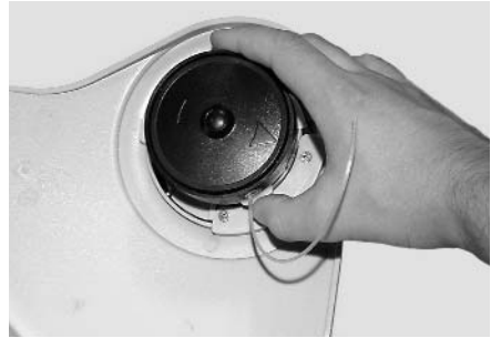
Figure 12. Manually advancing the cord
